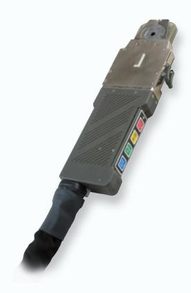
The MiniMicro™ weldhead was designed for precision welding of small diameter tubes and fittings. It is controlled by an orbital power-supply motor-control circuit to turn the rotor at the precise speed to create a near perfect weld.
