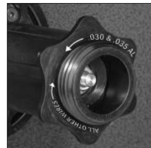
Wire Spool Retainer In "Tool Mode"; used to change spindle drag. Figure 3
