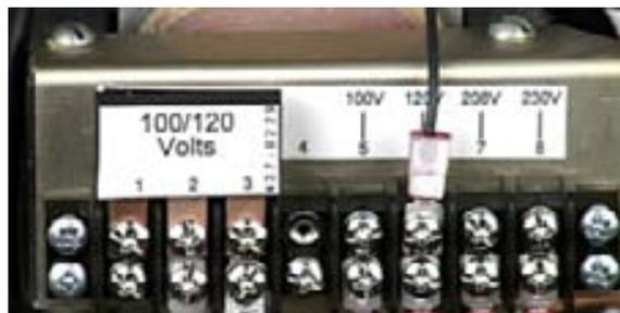
The CobraTig™ 150 can operate on any of four different input power values: 100VAC, 120VAC, 208/230VAC Single Phase and, 208/230VAC Three Phase. Attached to the unit is a 12ft power cable that comes wired from the factory ready for 120VAC. Even though the installed plug is only three prongs, there are four wires in the cable, ready for three phase power.
