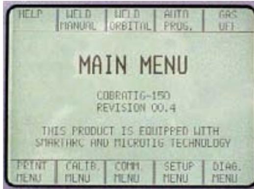
This is the starting menu for the CobraTig™ 150 orbital welder. It is from this menu that all the other menu displays and screens are accessible. From each menu display, there is a one-step button back to this menu.
