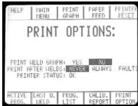
At the PRINT MENU, many different aspects of the CobraTig™ 150 can be printed or modified. Not only can various printouts of weld procedures, list of procedures, and calibration reports be made but the printer configuration can be modified to print on command or automatically.
