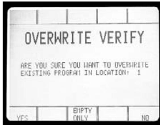
If the current procedure is to be saved at this location, press "YES". If this location is to be emptied, and the saved weld procedure erased, press "EMPTY ONLY". If nothing is to be done with this location, and you need to return to the SAVE PROGRAM MENU, press "NO".
