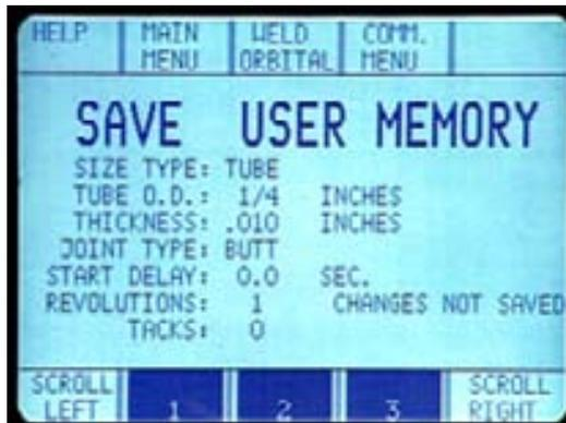
Once a weld procedure has been developed, it is generally a good idea to save it for use at a later date. In order to do this, simply press the SAVE PROGRAM button. This will change to the SAVE USER MEMORY screen.
