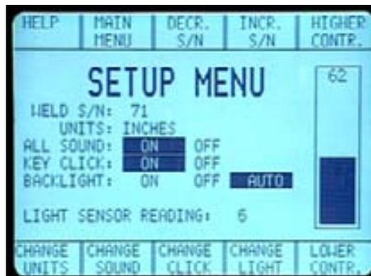
This menu is used to set up the user's preferences of the weld procedure serialization, button clicks and sounds, and LCD display contrast.
