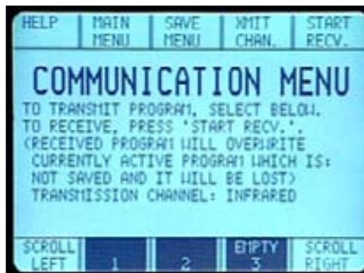
It is from this screen that weld procedures can be transferred from one CobraTig™ 150 unit to another. There are two paths available for transmission: IR (Infra Red) and Wired Cable. The IR method works much like a TV remote, just have the two units facing each other at a distance up to 10 feet and commence transmitting. While the Wired Cable is a cable hookup between the units' RS232 transmission ports on the rear panels.
