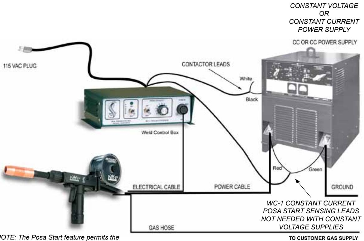
*NOTE: The Posa Start feature permits the WC-1 to be used in combination with any Constant Current DC power source with an open circuit voltage in excess of 55 volts.*
