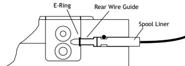
Remove both rear handle screws, and secure spool canister with longer screws provided.
