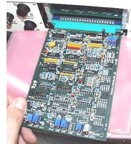
Connect Servo Board to card
