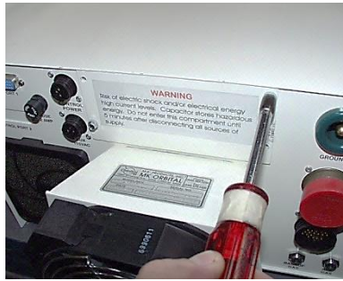
Removing Low Window Shield
