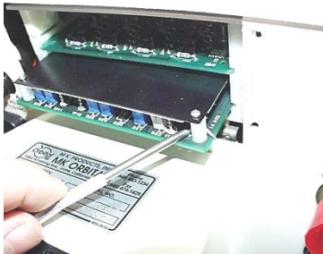
Remove Board with Hook
