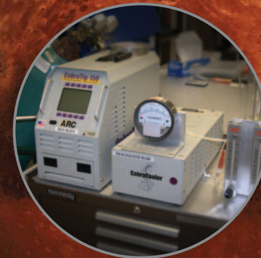
MK Products CobraTig Orbital welding system sits inside one of JPL's labs, ready to go to work. Image Credit: Doug Kensrue MK-JPL-1030
